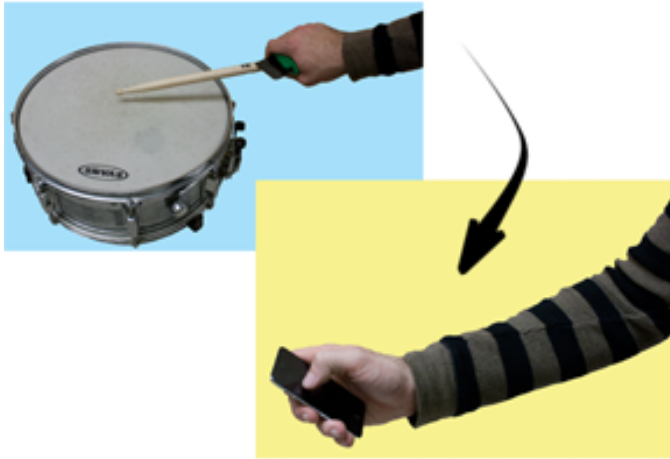
Fig. 2. The virtual percussion system aims to provide a experience that closely replicates an actual instrument. It was inspired by analyzing actual drum strokes and mapping features of the accelerometer signal to sonic qualities.
