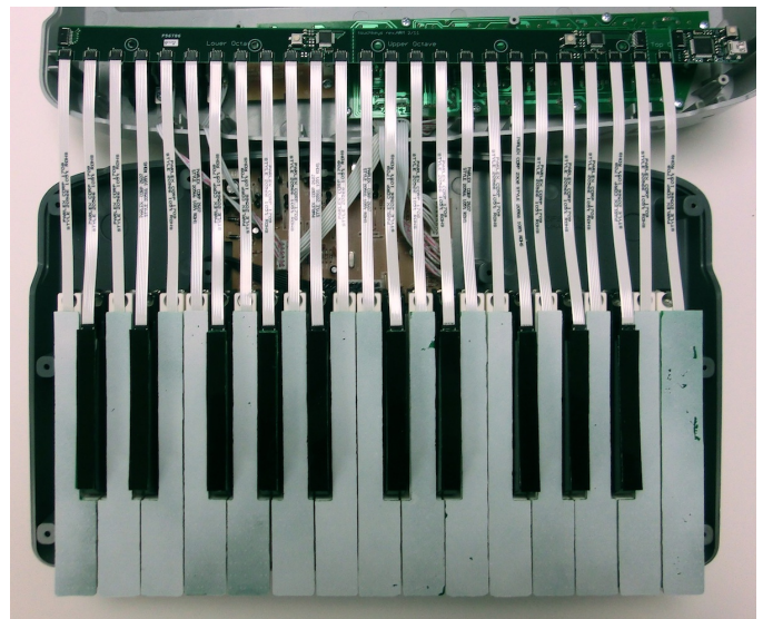
Fig. 6. Capacitive multi-touch sensors applied to a standard MIDI controller.
