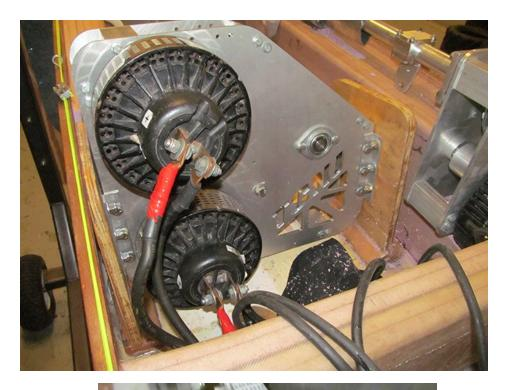
The dual inboard motors are driving the propeller shaft through high strength, notchbelt pulleys.
