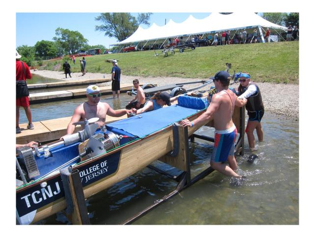
Launching the boat for a sprint event went off without incident. A sail cloth cover protected the motor controllers and batteries from splash, and a Go-Pro camera was mounted to the sprint motor assembly. The perforated metal cover over the belt and pulley mechanism was nothing more than a ventilated cover to keep fingers out.
