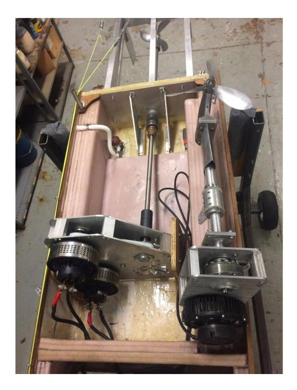
The entire onboard drive systems is shown above. The endurance motor bunk was eventually reversed in order to move the center of balance aft. Notice that the endurance power unit is also notch belt driven. Both propellers were designed and machined in-house.
