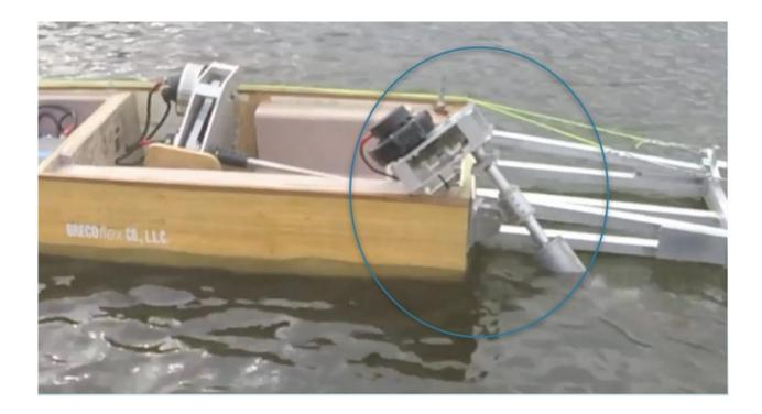
Although tilting the endurance outboard motor was the original plan, it became obvious that the unit could not be raised completely out of the water. Even reversing the motor on the powerhouse was still not enough. The foam bunk was then fabricates to store the endurance outboard within the hull during the sprint events.
