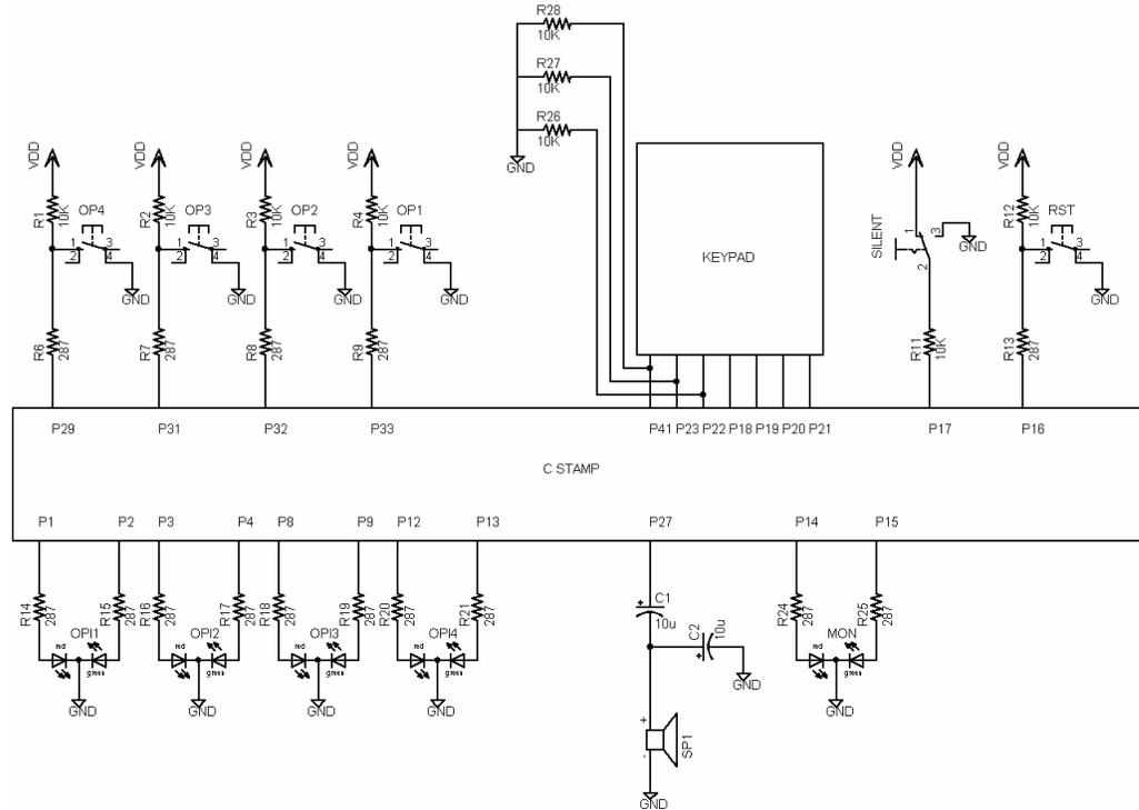
For this project, we simulate the four openings being monitored with four push-button switches OP1 through OP4, and their associated resistors. This represents a monitoring scheme with a normally open contact and pulled **HIGH**. This means that when an opening is closed, there is a contactor that is open, and when the opening closes, this contactor closes and the C Stamp pin monitoring the opening is pulled
