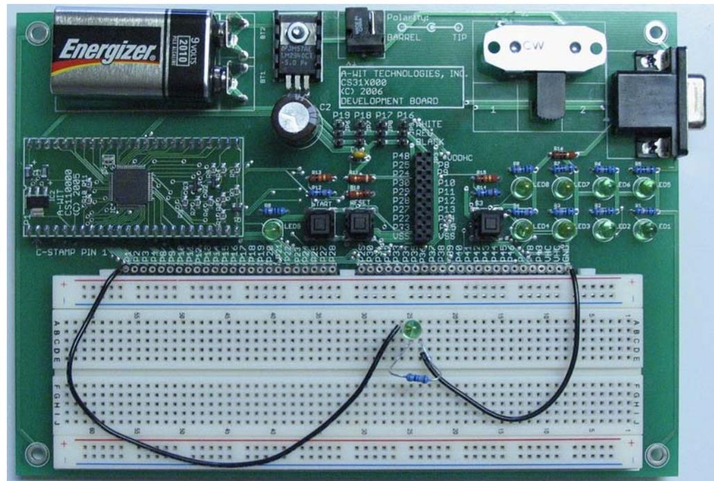
The programming problem at hand is to turn the LED on and off 60 times in one minute or every second. The program below will accomplish this task. As is the case in programming, there are multiple solutions to a programming problem. The code below is our solution, and the comments embedded in the code offer more clarifications.
