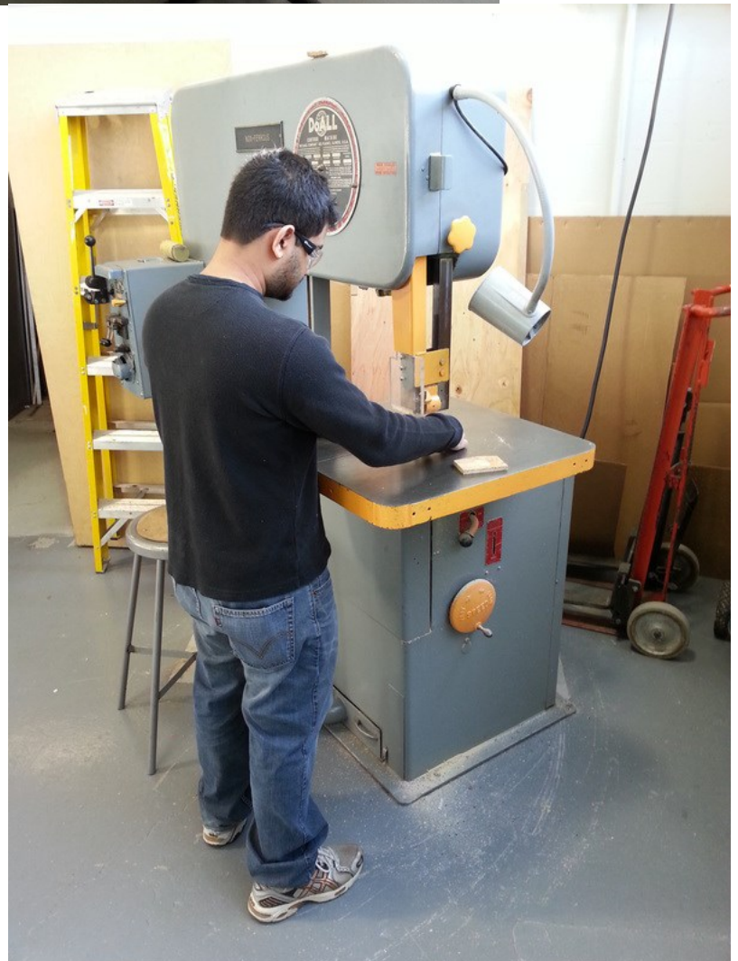
Above, Kyle, Brian, and Manthan layout rib stations to be used in building the hull plugs. At the right, Manthan simply cuts out the 5/8 inch OSB stock for each rib.
